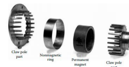
FIGURE 7.26 Claw poles with PM. (From Pavlak, A.M., Proceedings ICEM '92 International Conference on Electrical Machines , Vol. 1, University of Manchester Press, 1992. With permission.)
